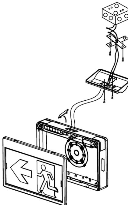
3. Reference step 3 - 5 in wall mounting above for ceiling mounting.
