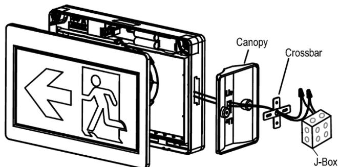
3. Reference step 3 - 5 in wall mounting above for side mounting.
