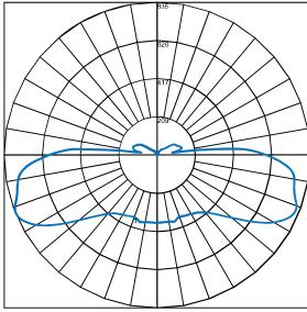
Maximum Candela = 834.97 Located At Horizontal Angle = 225, Vertical Angle = 68 # 1 - Vertical Plane Through Horizontal Angles (225 - 45) (Through Max. Cd.)
