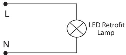
Easy to install - bypass ballast and provide voltage directly to lamp
