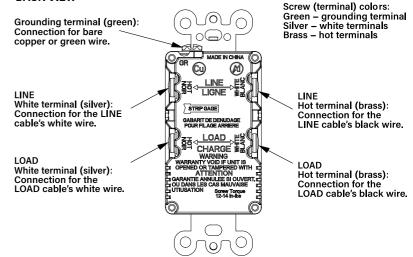
Maximum tightening torque 14in-lbf(1.6N.m)
