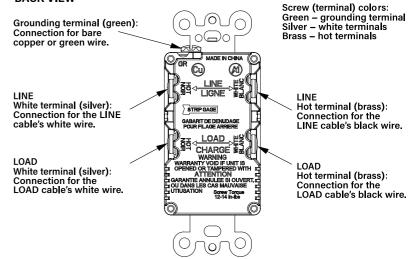
Maximum tightening torque 14in-lbf(1.6N.m)
