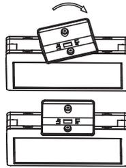
Insert canopy into housing at 20 degree angle and twist. Quick snap is now firmly locked.
