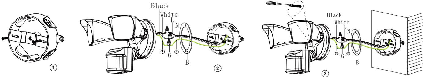
1. Fixing the bracket installation hole with junction box hole by screw, the screw included in accessory bag.
