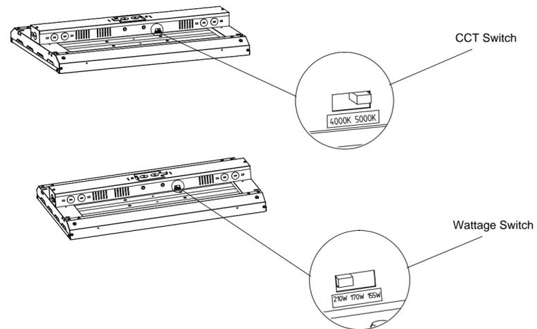
The end users may adjust the color temperature and lumen output respectively by the two DIP switch. The power switch has three options (left, middle and right), and the color temperatures switch has two options (left and right), corresponding to three powers and two color temperatures respectively, which can perform the desired color temperature and lumen output combination.
