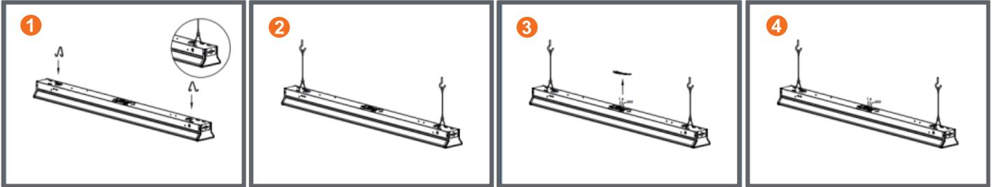
1. Install the hanging hooks(included)onto the top of the fixture,Make sure the wiring hangers are fully engaged into the holes on the top channel.
