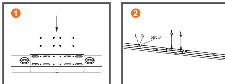
1. With screws,Use the connecting fittings to lock the back of the fixture.
